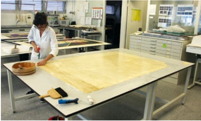
Figure 13. Lining of the posters with Japanese paper. The sheets of Japanese paper are being prepared on the lining base.
