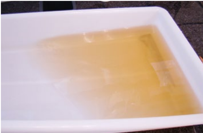
Figure 9. After the washing, soluble degradation by-products are washed away from the sheet. After the wash, the water becomes yellowed and acidic.
